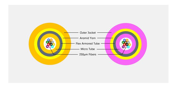
Codecom Indoor / Outdoor Microcore Flex Armoured fibre cable contains up to 24 fibres of 250µm in a micro tube.
